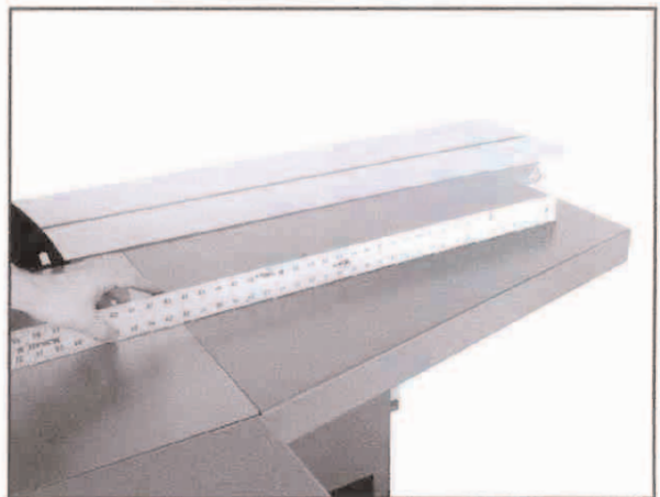
Figure 22. Checking with a straightedge.
