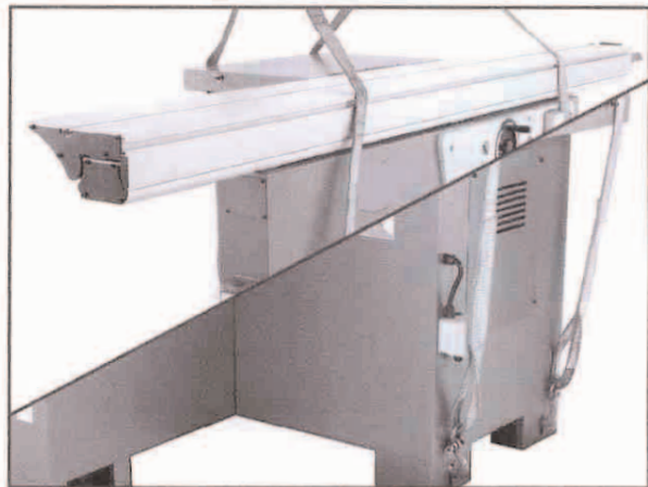
Figure 17. Lifting the saw base unit.
