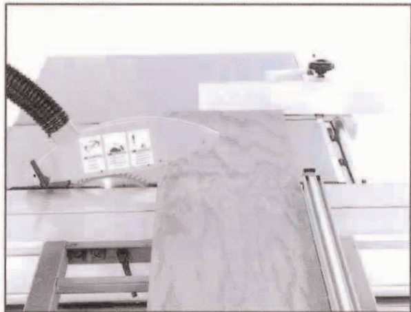
Figure 61. Correct rip fence position when using it as a cut-off gauge.
