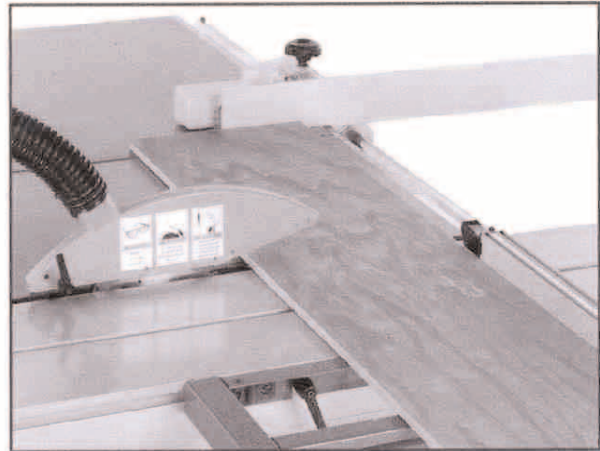
Figure 59. Crosscutting workpieces using the rip fence as a cut-off gauge.
