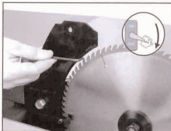
Figure 34. Adjusting the riving knife.
